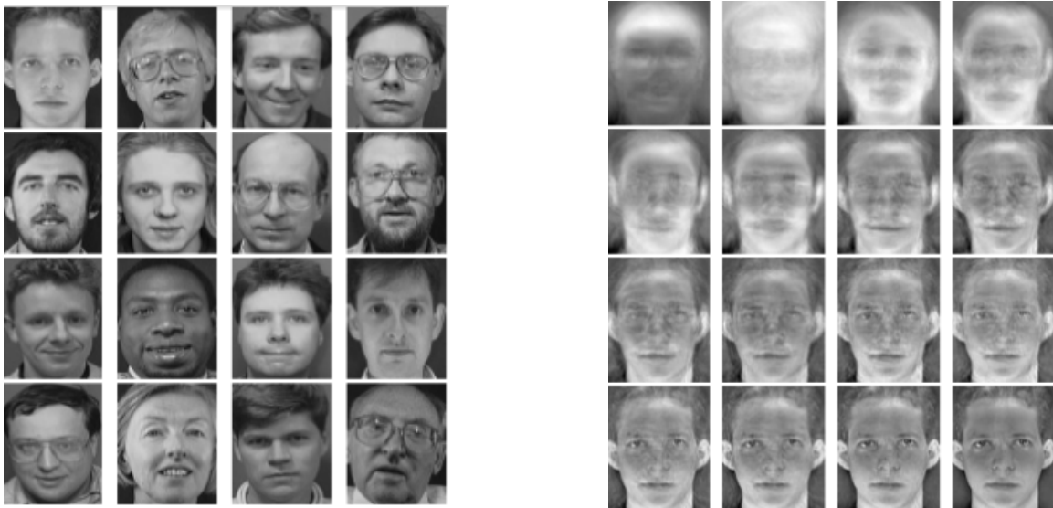
Figure 2: On the left, samples of grayscale, 100 \times 100 pixel images of human faces. On the right are the first sixteen eigenvectors generated using PCA successively added together to recreate a face. [5].
